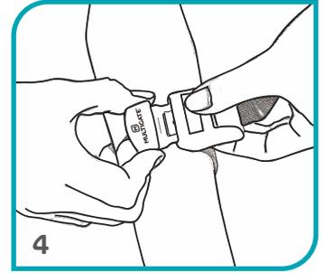
For a quick release, press the top smooth button on the buckle.
